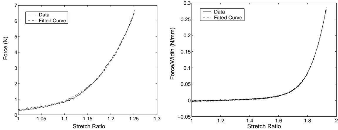
Figure 3. Plots of in-vivo (left) and ex-vivo (right) measurements of porcine small intestine. The width of the ex-vivo sample is 15mm. The in-vivo measurement is performed with an 8mm wide babcock gripper.
