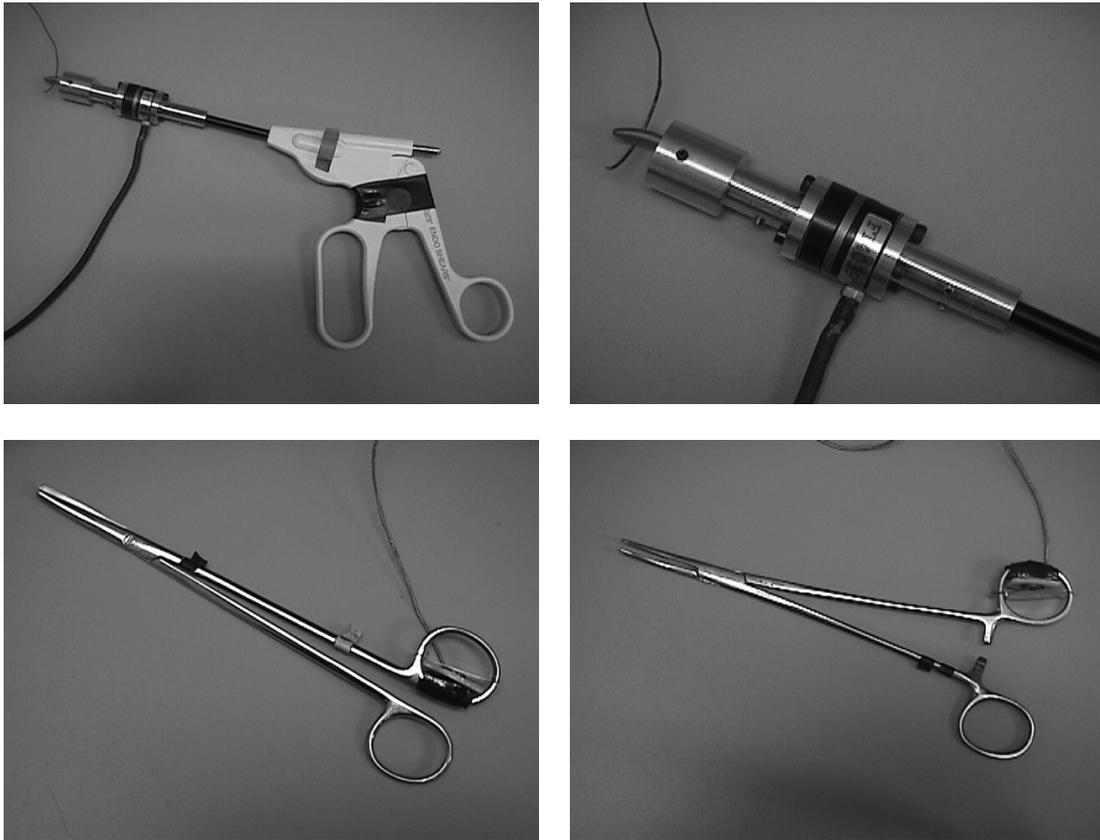
Figure 2. Force sensors mounted on surgical instruments. Top: 6-axis force/torque sensor on adapted grasper (left); close-up of sensor attachment (right). Bottom: load cell mounted on scissors (left) and clamp (right) to measure cutting and spreading forces, respectively.
