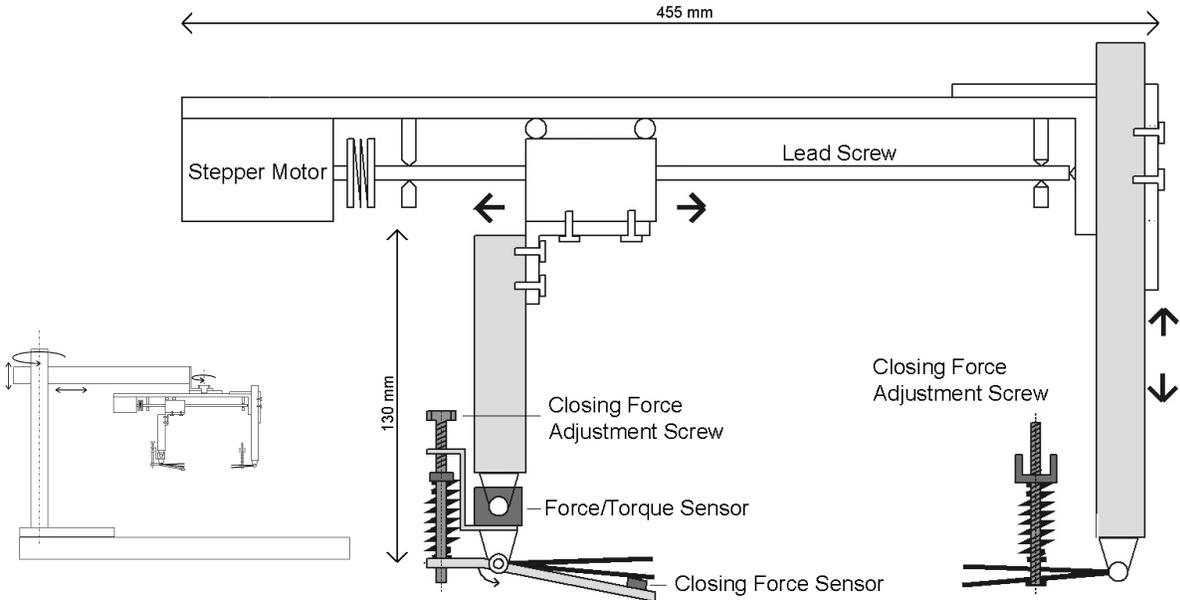
Figure 1. The instrument used for uniaxial stretching experiments in-vivo and ex-vivo. Inset shows how the device mounts on the operating table.
