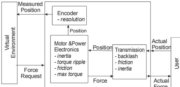
Figure 5. Flow diagram of forces and positions in a virtual reality system with haptics, and the factors that limit haptic fidelity.
