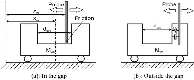
Figure 3. Schematic representation of the backlash model in a single translation
