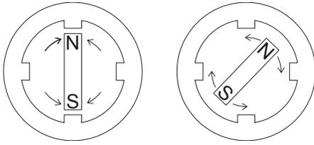
Figure 4. Cogging: A stable (left) and unstable (right) detent position of a permanent magnet (brushless) motor. A fluctuating torque can be felt due to the magnetic attraction between the permanent magnet rotor and stator teeth.
