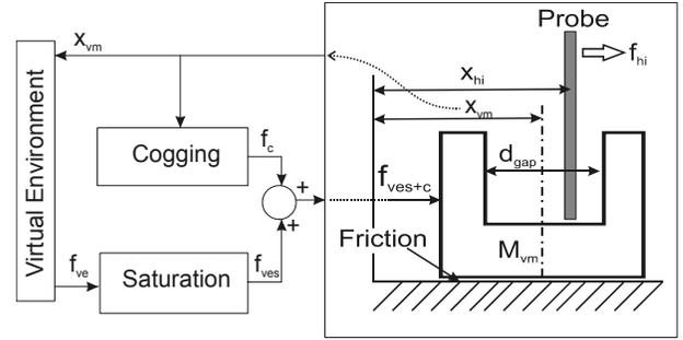
Figure 6. The basic physical representation of our model integration.
