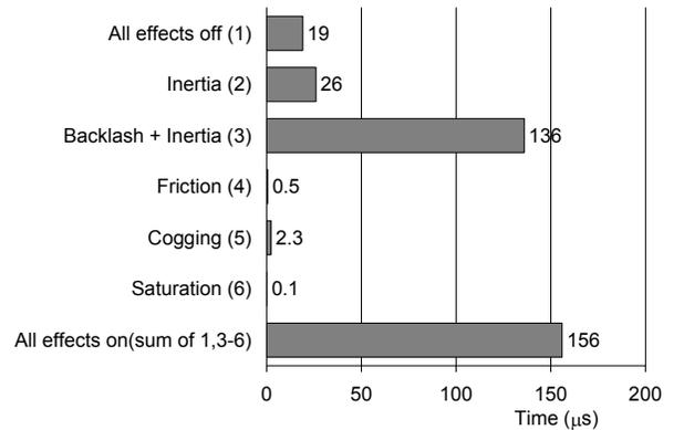
Figure 10. Chart with computing times of the various degradations.
